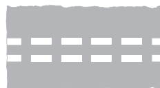
Give way to traffic on major road (can also be used at mini roundabouts)
