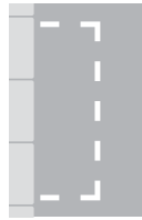
Waiting is limited to the duration specified during the days and times shown
